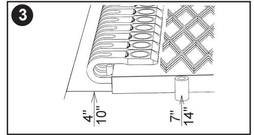
**3.** Insert belt in fastener strip against belt stops and belt edge stop pin for 7" and 14" belts. For 4" and 10" belts, align belt edge with line.
