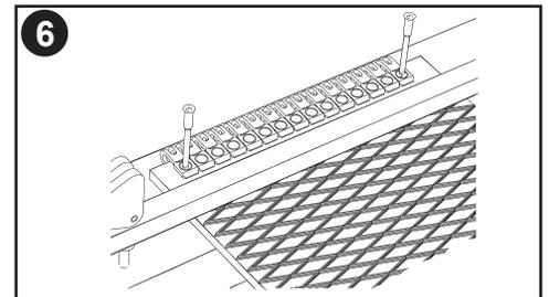
**6.** Using a 1-pound hammer, drive a rivet through the hole in the last fastener at both ends of the fastener strip. Do not final set rivets.
