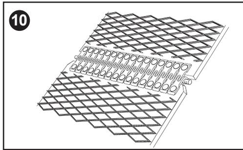
10. Notch trailing edge of belt on both sides. Bring belt ends together and insert corrugated pin. Remove nails from the tool.
