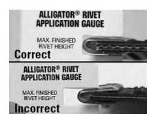
How do you know when the fastener is installed correctly? Installing Alligator® Rivet requires striking the fastener strip several times with a 1 lb. hammer. The gauge should easily slide onto your fastener strip after installing. If the gauge does not slide over each plate the fastener strip needs to be placed in the tool and struck several more times to ensure proper compression.
