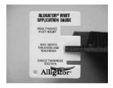
How much impression top do I remove? The gauge will tell you when you have removed enough impression top to allow proper installation of the Alligator Rivet fastener. When the gauge can be placed on the belt and can slide across the width without encountering resistance the belt has been properly skived. If the gauge cannot be inserted onto the belt then additional impression top must be removed.
