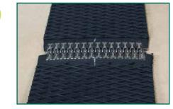
To join ends, connect the fasteners with the correct offset so that the belt edges line up.
