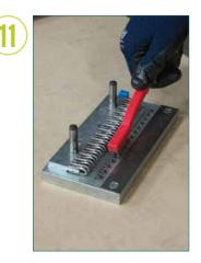
After each installation, remove any trapped rubber particles from the tool using a small wire brush.
