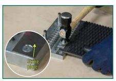
Flatten the rivets on the reinforced strike plate. Do not strike or damage the loop area of the fasteners! (*Tip: use the peen on a ball peen hammer to flatten rivets*).
