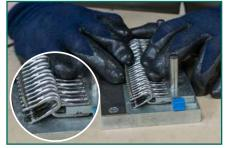
Insert fastener strip into the tool. Make sure the fastener strip is properly placed with the pins resting in the recesses of the fastener. (*Tip: load the back of the plate first, then swivel the loops down and into place*).
