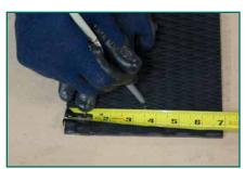
Mark the belt ends for fastener positioning. Place a mark 1.5mm (1/16") offset from the centerline on both belt ends toward the same side of the belt.
