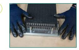
Insert belt into the fastener strip and against the belt stops. Align the center of the fastener strip with the offset mark on the belt end. (*Tip: pre-mark the tool's fastener holder for the center of frequently used widths of fastener strips*).
