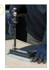
Use a 1/2 pound hammer to set the rivets (do NOT use a pneumatic hammer). Follow the sequence shown for the first three fastener segments. Continue to set the remaining rivets in any sequence. (*Tip: be sure all rivets* have been set prior to removing the splice from the tool).
