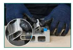
Insert fastener strip into the tool. Make sure the fastener strip is properly placed with the pins resting in the recesses of the fastener. (*Tip: load the back of the plate first, then push the loops down and into place*).
