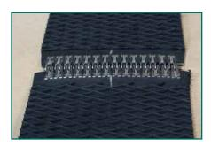
To join ends, connect the fasteners with the correct offset so that the belt edges line up.
