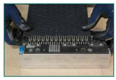
Insert belt into the fastener strip and against the belt stops. Align the belt's center line with the appropriate selection on the sticker. (Tip: the number of fasteners on the selection sticker refers to the segment count. Example: a seven inch wide belt requires a fastener strip with 14 segments).
