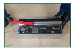
After each installation, remove any trapped rubber particles or debris from the tool using a small wire brush.
